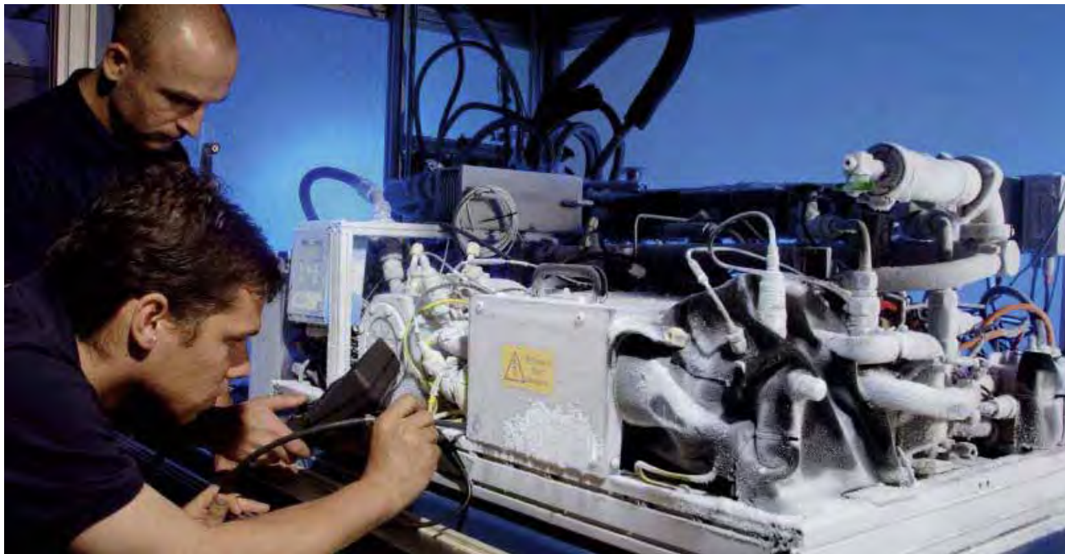
Test of the fuel cells' cold-start capabilities in the climate chamber.
