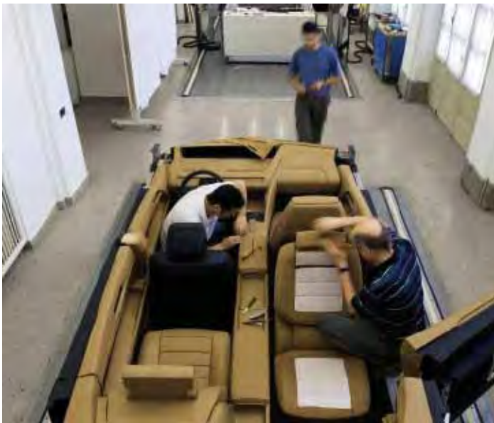
Using a 1:1 clay model, the designers can see what the interior of the F 700 will look like with a REVERSE seat.
