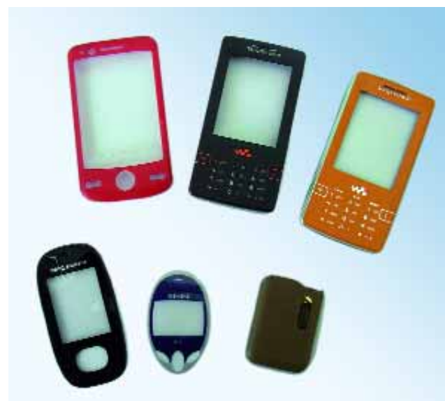
High quality effects of finishes with decor films – In Mould Labelling (IML) at the Balda location in Xiamen, China
