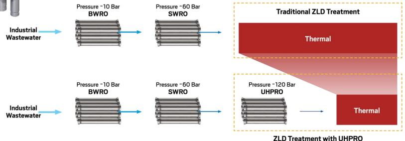
Applying UHPRO to ZLD treatment reduces thermal requirements at the end of the process
