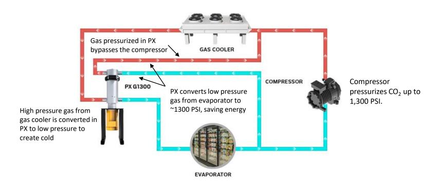
We have expanded the aperture of the PX technology to successfully compress gas, allowing for efficient energy transfer in refrigeration
