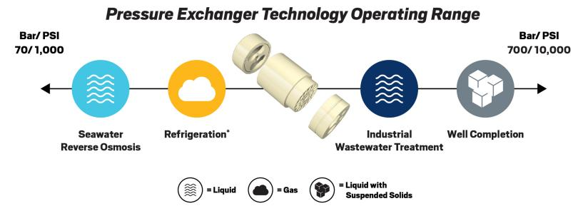
\*Pressure Exchanger in refrigeration can handle multiple phases of CO2(liquid, gas, and supercritical fluids)
