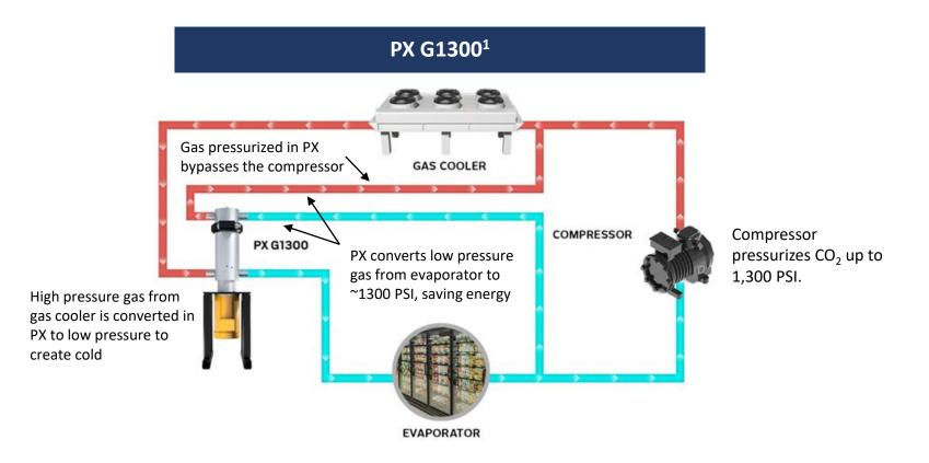
We have expanded the aperture of the PX technology to successfully compress gas, allowing for efficient energy transfer in refrigeration
