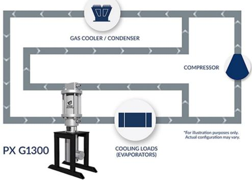
\* Low pressure CO<sub>2</sub> is simultaneously routed to a compressor and the PX G1300 which allows the customer to reduce the compressor size. Refrigeration system gas process flow diagram incorporating our PX G1300 is for illustration purposes only. Actual configuration may vary.
