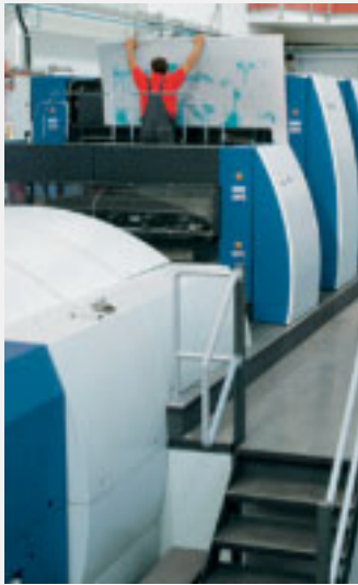
Superlarge sheetfed offset presses for a sheet size of 1510mm x 2050mm are a KBA world exclusive
