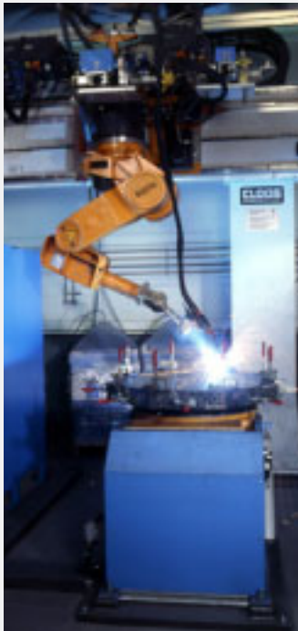
Welding robot in action in the sheet metal production line at our Würzburg facility
