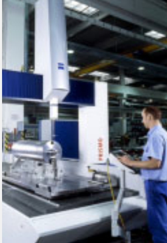
ISO 9001 quality inspection at a cylinder using a high-tech measuring machine
