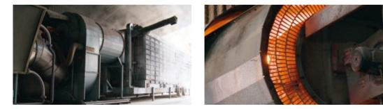
FLUE GAS-FREE DRYERS PROVIDE QUALITY AND ARE OPERATED WITH ECO-FRIENDLY ENERGY FROM OUR BIOGAS PLANTS.
