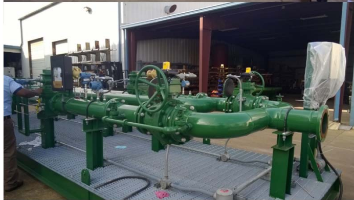
LACT units fabricated in Sugarland, Texas (USA)
