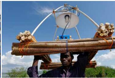
When the battery needs to be recharged or exchanged at the energy hub, customers are charged around one euro. Compared with the 1.5 liters of kerosene (costing around €1.50) that are used for each night's fishing, charging the battery cuts costs by a good third.
