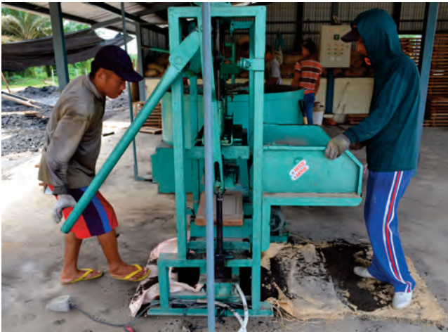
Production of building bricks
