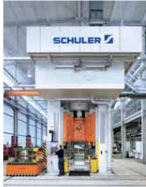
Hydraulic drawing press for the production of boiler parts
