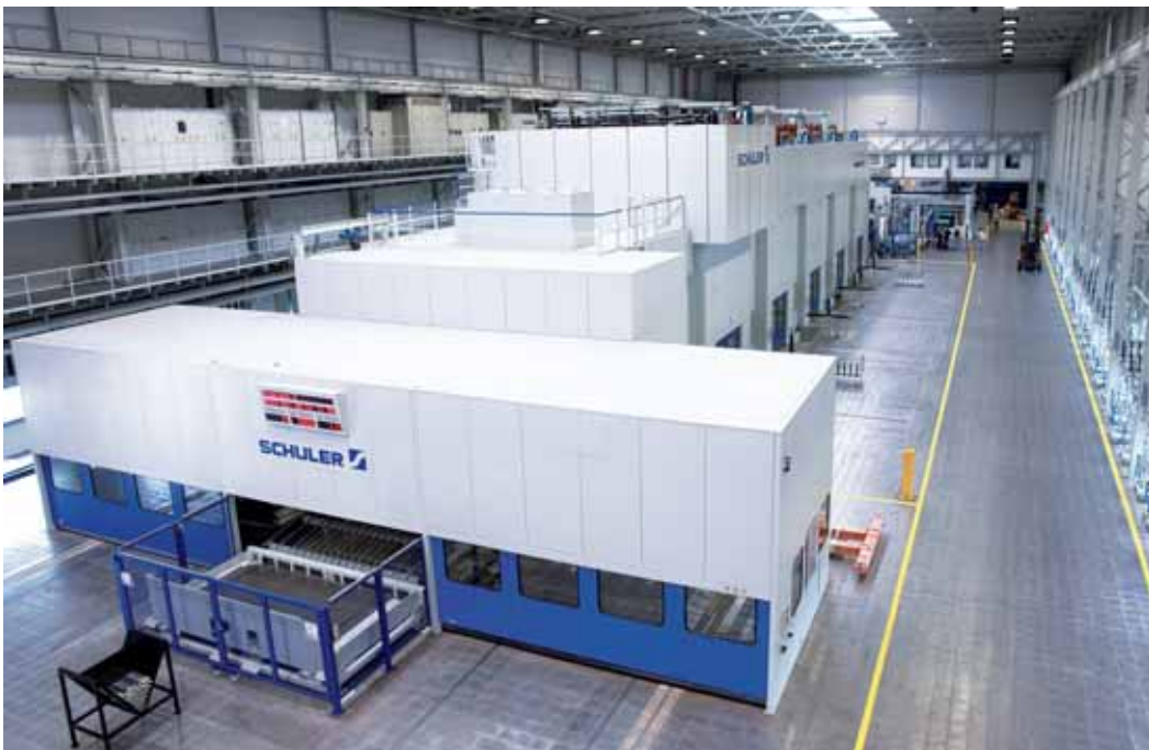
Hydraulic press line with blank loader (in the front) and robot automation
