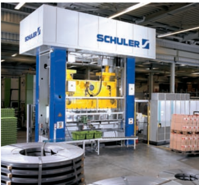
Blanking and forming press with servo drive automated with coil line and feeder. Maximum press force: 400 t
