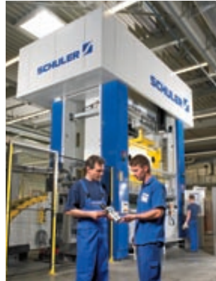
Blanking and forming press with servo drive (press force 400 t)
