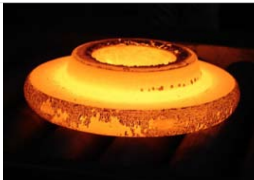
At 1,200 °C, ring blanks are manufactured on the Schuler press
