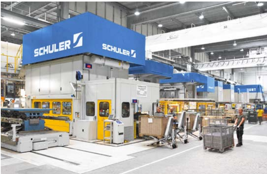
Cookers and cooktops are manufactured on the 800 t platform press (see page 15)
