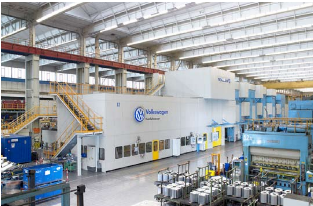
High quality, flexible, fast – almost all of the new Porsche Panamera's body panels are produced on a hydraulic press line
