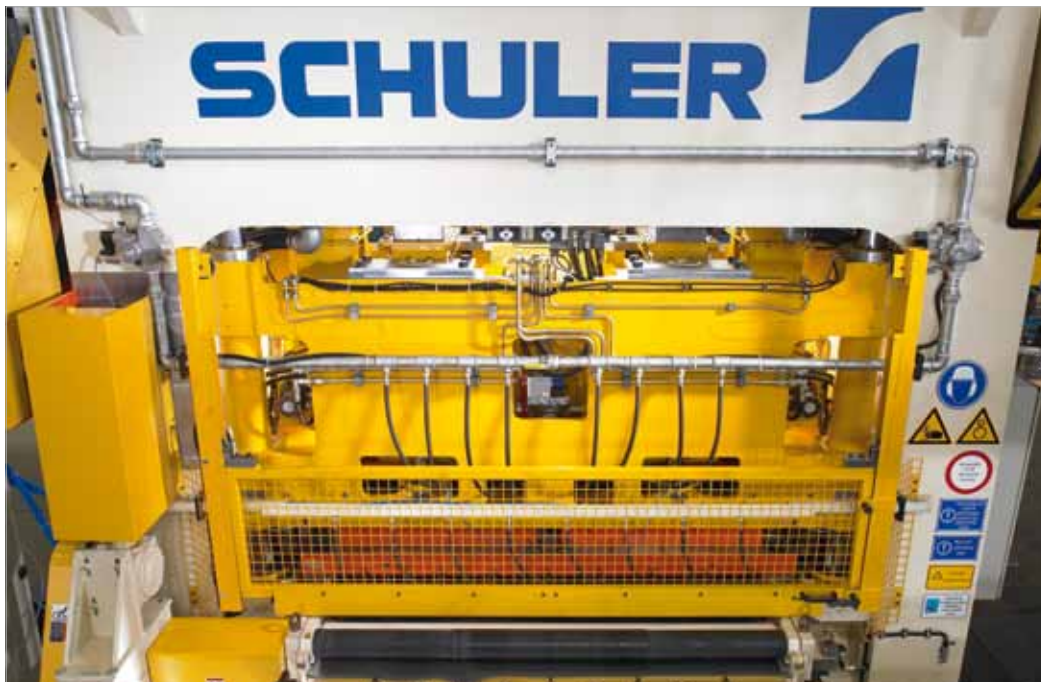
Schuler cupping press for the packaging industry: the welded monoblock body with play-free preloaded slide guidance system ensures precise slide movement
