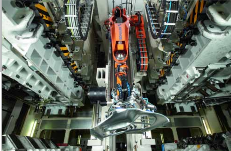
Schuler's Crossbar Feeder guarantees safe part transport along BMW's servo press lines
