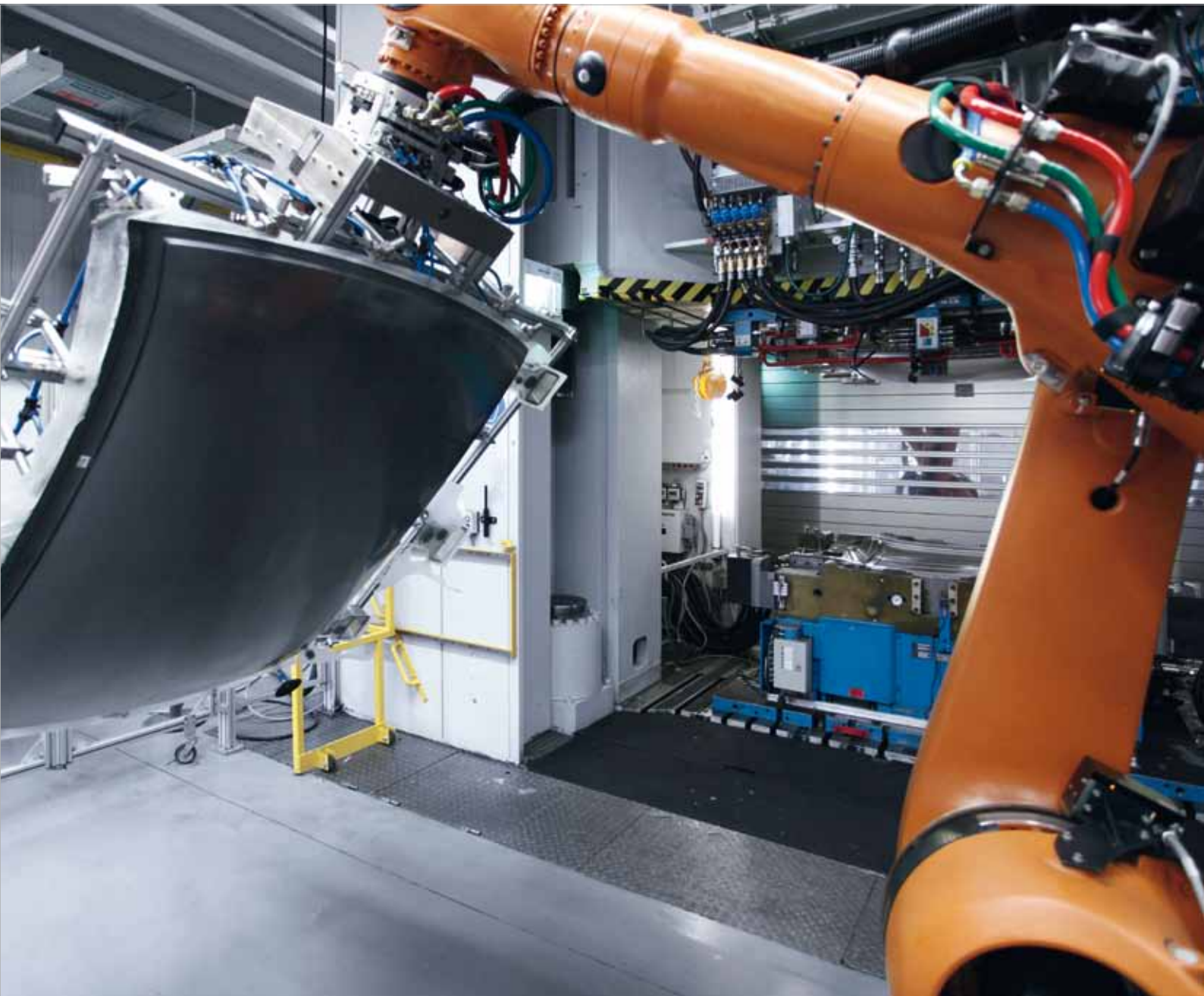
Removing a carbon roof from the composites press
