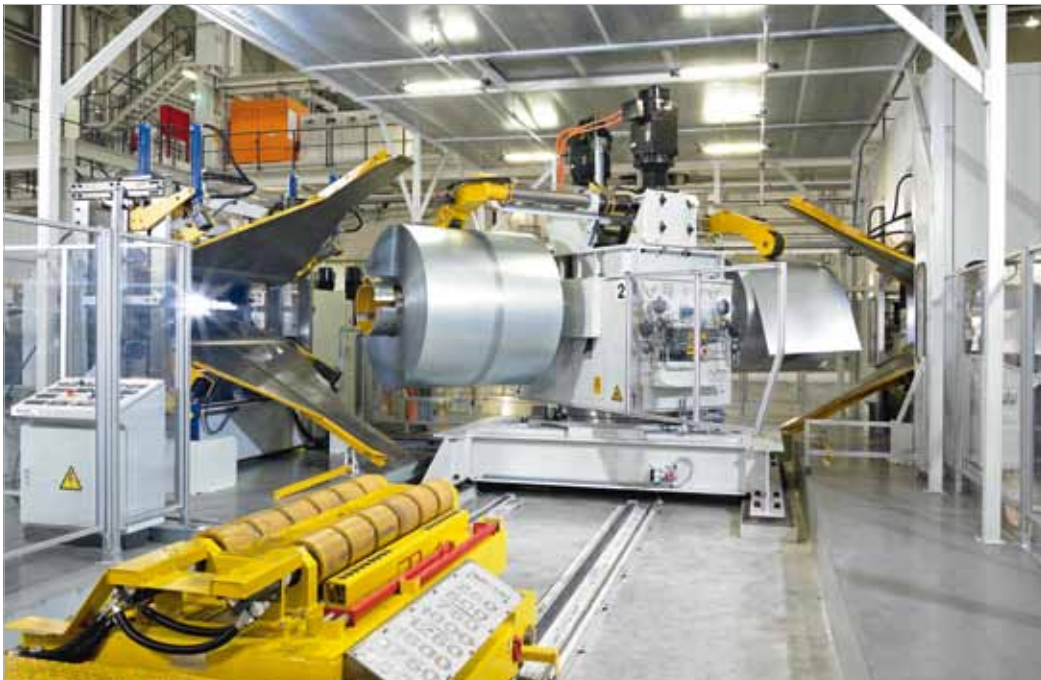
New Schuler cutting line with ServoDirect technology for optimizing coil preparation at BMW
