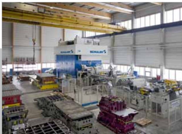
Tie rod construction servo press with coil line and blankloader from Schuler
