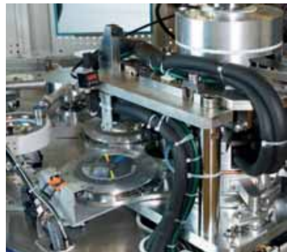
Embossing unit in a BLULINE II production system for 50 gigabyte Blu-ray Discs
