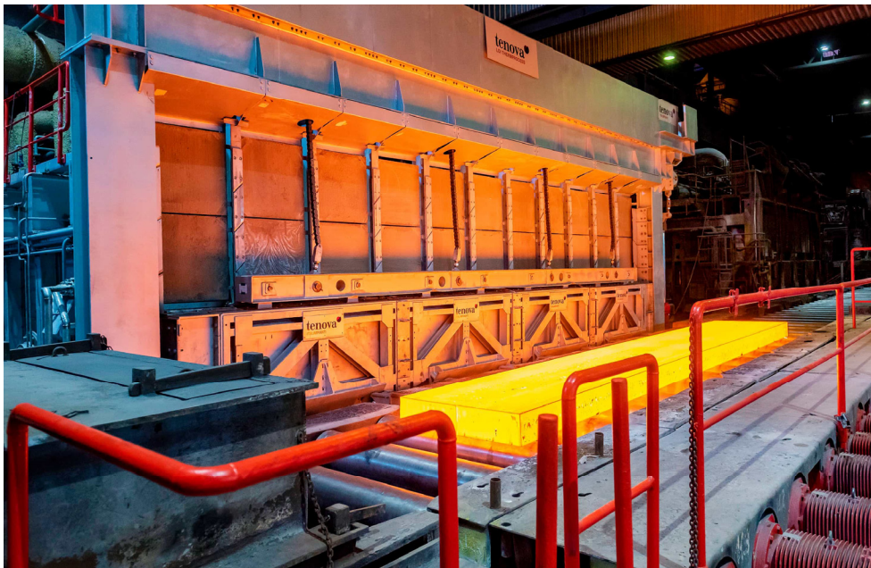
The new walking beam furnace in Duisburg heats slabs gently to avoid surface damage.
