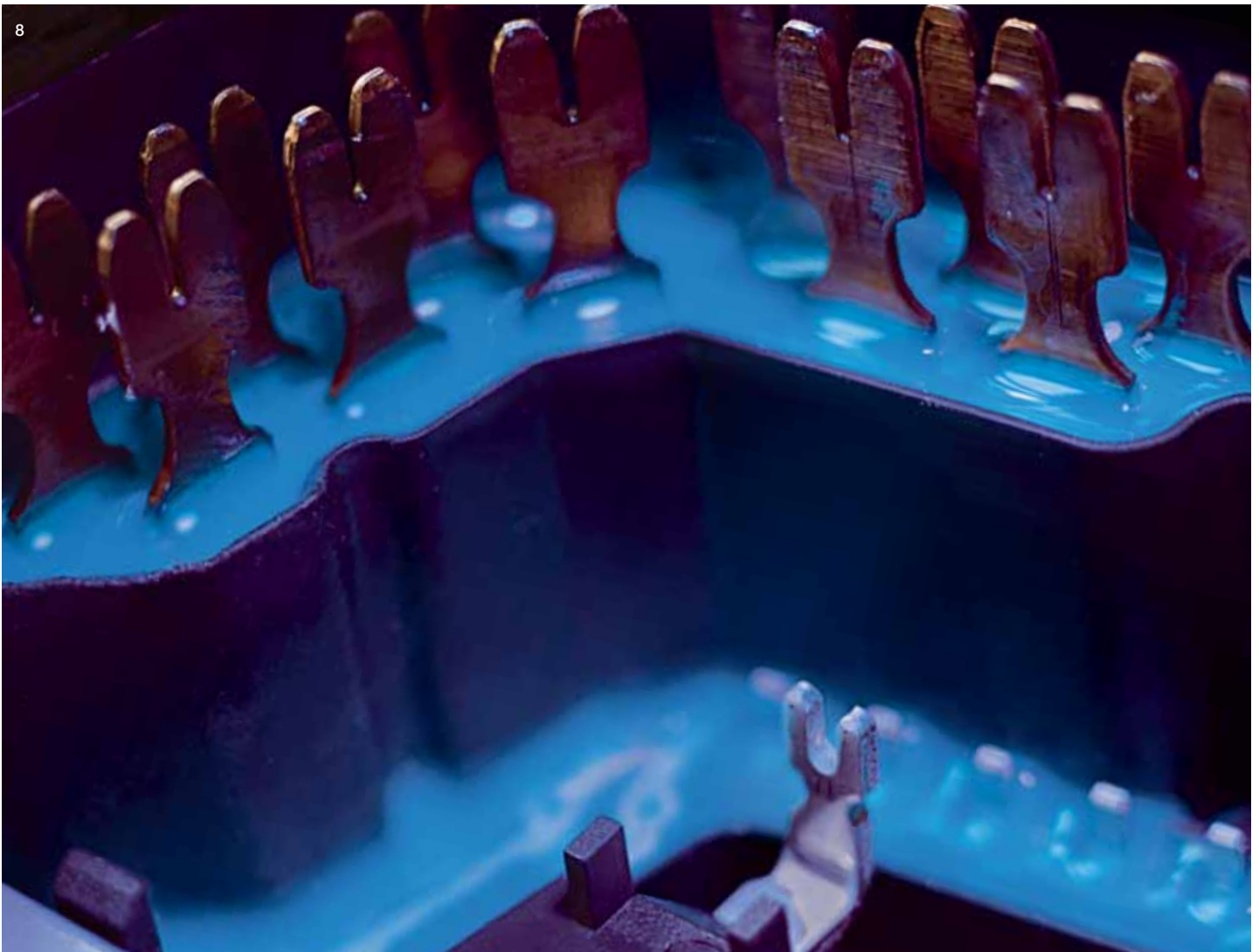
6 A few drops are enough: a pressure sensor is encapsulated with SEMICOSIL® fluorinated silicone gel.
